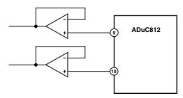
Figure 22. Buffering the DAC Outputs
